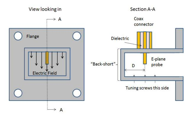
The coax is typically 50 ohms impedance, whereas the waveguide might be 200 ohms. Actually, the impedance of waveguide is a complicated subject, there are three ways to calculate it, and it is a strong function of frequency. Therefore, some tuning must be applied. The tuning can be in the form of screws, or position of the probe, or the distance to the back short.
